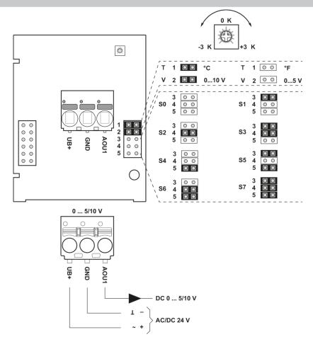
the adjustment of the measuring ranges is made by changing the bonding jumpers the output value in the new measuring range is available after 2 seconds Setting range I°C1 range I°E1 Eactory
